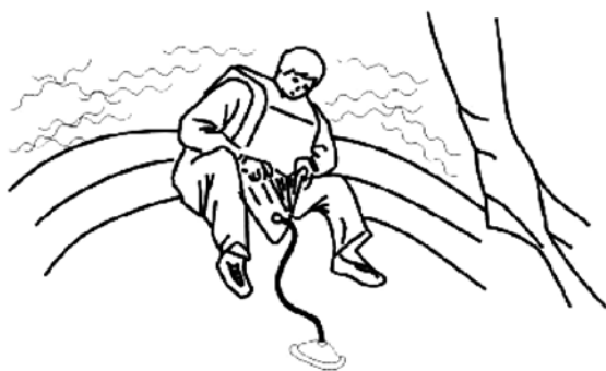
Picture 15 Inflate Floor (if inflatable) with Bellows
