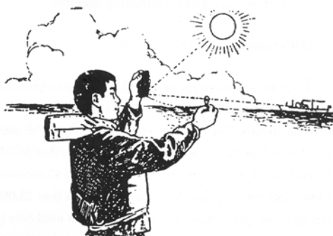
Figure 24 How to use the heliograph
