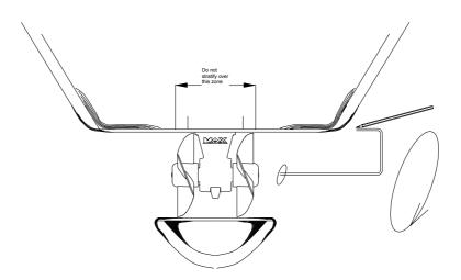
Fit the tunnel and mark the areas to be fibre-glassed. Sand these areas inside and out. In certain installations it is preferable to drill the position of the thruster support before the installation of the tunnel.
