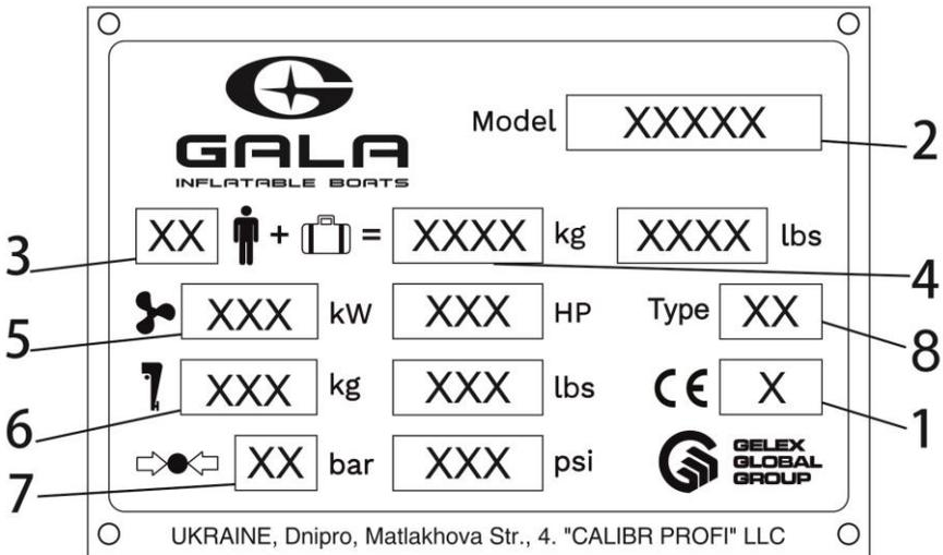
The indications on the capacity plate give information about limitations imposed by international regulations. Your local regulations can be different. Also these indications are not a complete list: the security requirements (obligatory security equipment of the boat, maximum authorized distance you can navigate from a shelter, etc. ) may change according to the country or state.
