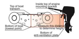
**Motor adjusted too low** : loss of speed and more difficult steering may occur (splashes). b) Motor trim:
