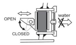
Inflation-deflation valve has PUSH- PUSH operating system: pressing the central pin the valve switches between OPEN and CLOSED. To inflate the tube put the pin to CLOSED position (pin moves UP). To deflate the tube put the pin to OPEN position (pin moves DOWN). After inflation every valve must be closed with the valve plug tight to ensure airtightness of the tube.
